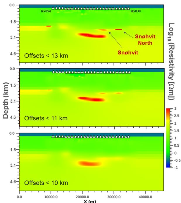
**Figure 2:** Resistivity section obtained by 2.5D inversion over the Snøhvit field using different range of offsets. Including offsets  $> 10$  km into inversion is crucially important for imaging both compartments of the Snøhvit prospect.
