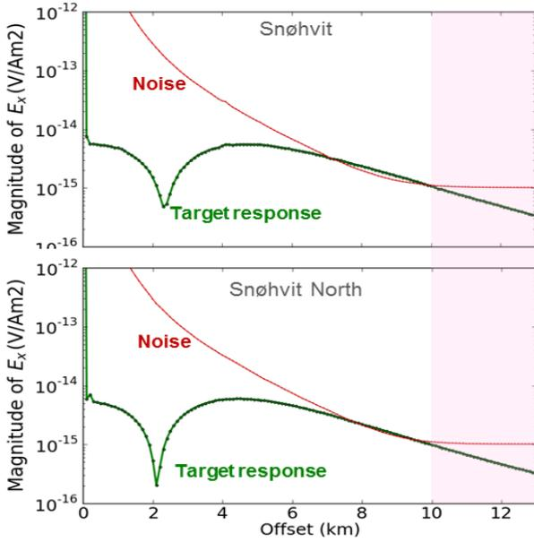
**Figure 4:** Green curves: Scattered field from a resistive reservoir: Snøhvit (top) and Snøhvit North (bottom). Red curves: noise level. For offsets  $> 10$  km the scattered field is below the noise.
