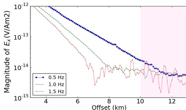
**Figure 3:** Magnitude versus offsets curves for inline electric field for receiver Rx036 for three frequencies. Data in the shaded region  $> 10$  km proved to be critically important for inversion despite they are strongly affected by noise.
