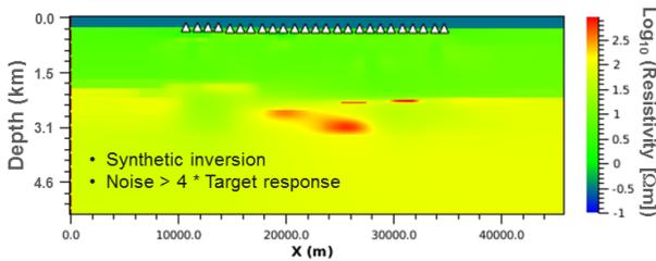
**Figure 6:** Both target resistors are well resolved by inversion of synthetic data contaminated with noise which is at least two times above the target responses
