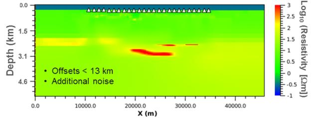
**Figure 5:** Inversion results like in Figure 2 (top), but the real data were contaminated with additional noise whose magnitude exceeds the CSEM response for both resistive targets.
