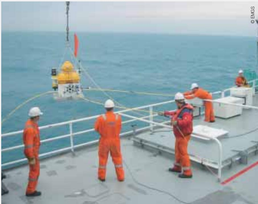
The receiver measures the electrical and magnetic fields generated by the source and which have travelled through the ground.
