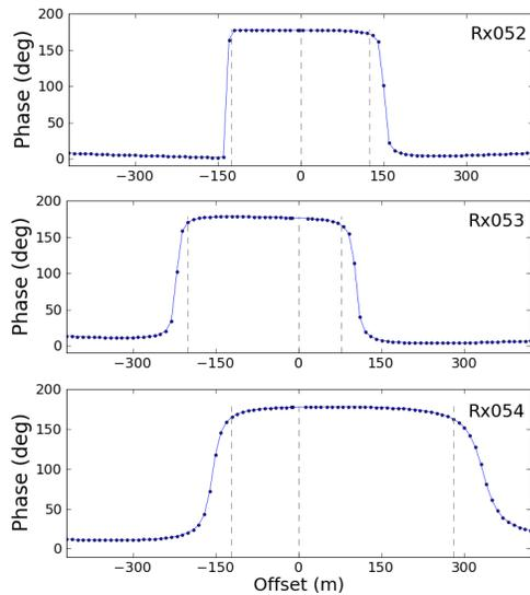
Figure 2: Short-offset PVO curves used for data QC for receivers marked in Figure 1. Receiver Rx052 on fairly flat seabed: symmetric PVO. Receivers Rx053 and Rx054 on the opposite slopes of a trench show asymmetric PVOs shifted towards the trench center. Frequency: 0.15 Hz.
