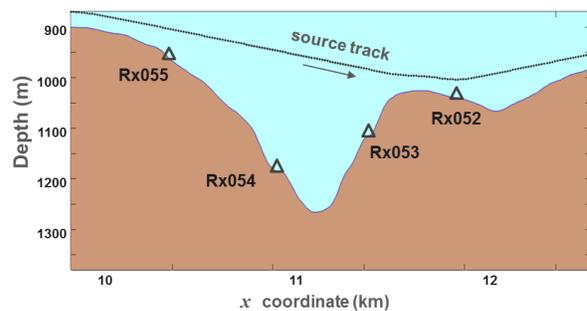
Figure 1: Seabed geometry, CSEM source trajectory and receiver positions (triangles) for a CSEM survey offshore Brazil.
