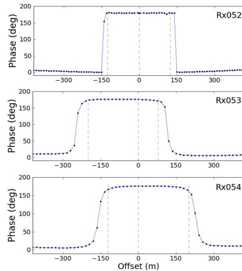
Figure 3: Synthetic PVO curves computed using bathymetry from the real survey for the same receivers as in Figure 2. Synthetic results reproduce very well the asymmetry of the phase flips in the observed data for Rx053 and Rx054.
