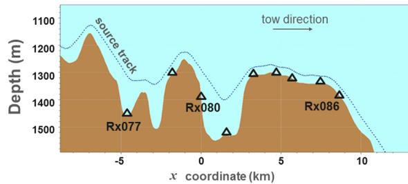
Figure 4: The rough bathymetry profile, receivers (triangles) and CSEM source trajectory from a survey offshore Brazil. Receiver Rx080 is located at the steepest part of the trench slope.
