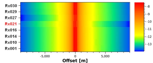
Figure 7: Synthetic MVO data,  $\log|E_{in}|$  at 0.1 Hz, computed using the model from Figure 6. Data for receiver Rx021 located on the trench slope shows a strong reduction in the magnitude on outtow and an increase on the intow, as compared to other receivers. These are the same trends as for real data of Rx080 in Figure 5.
