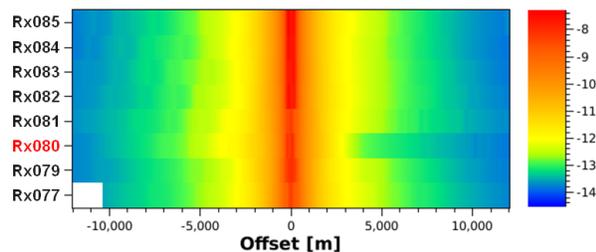
Figure 5: MVO data for the inline electric field  $E_{in}$  at 0.12 Hz for several receivers, the color scale indicates  $\log|E_{in}|$ . Data for Rx080 located on a trench slope (see Figure 4) has anomalously low magnitude on outtow and higher magnitude on intow.
