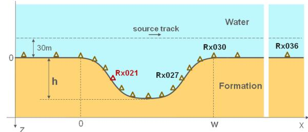
Figure 6: Bathymetry profile, source trajectory and receiver positions used for a synthetic study of the trench effect. Data for receiver Rx021 turned out to be most affected by the presence of the trench.
