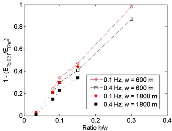
Figure 8: Reduction of the inline electric field for receiver Rx021 on a trench slope compared to a reference receiver, plotted as a function of the trench depth/width ratio.
