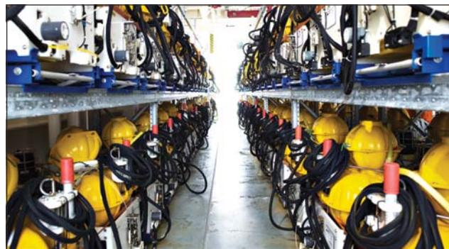
**Figure 2** Up to 200 receivers can be kept aboard EMGS's high-capacity 3D EM surveying vessels. More receivers means larger and more complex surveys, and more data points per km<sup>2</sup> for improved 3D data coverage.
