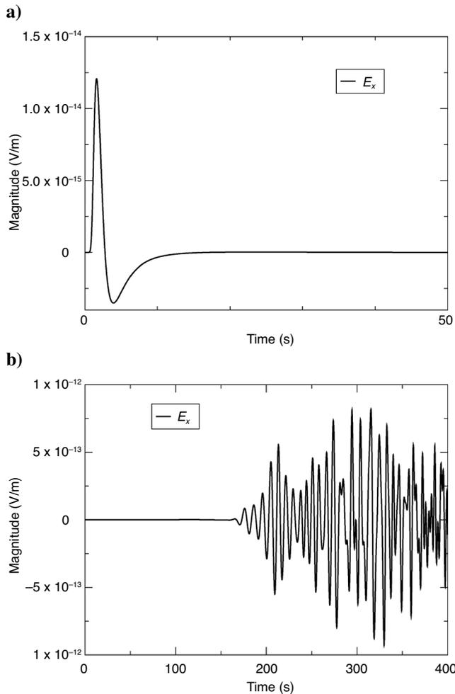
Figure 2. Resulting time series for the inline electrical component  $E_x$  at 10-km offset using (a) the standard method and (b) the proposed method.
