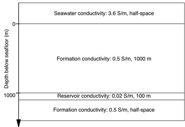
Figure 1. The plane-layered model used for comparison of results. The model consists of a semi-infinite water layer, a 1-km formation layer, a 100-m resistive layer, and a semi-infinite formation layer.
