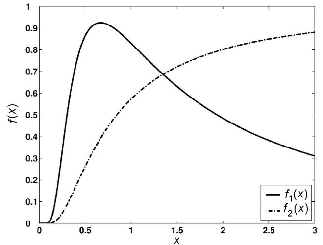
Figure 3. Step responses for dipole radiation in conductive materials: far-field response  $f_1(x)$  (solid line) and near-field response  $f_2(x)$  (broken line). The far-field response is largest for  $x < 1.4$ .
