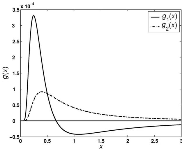
Figure 4. Impulse responses for dipole radiation in conductive materials: far-field response  $g_1(x)$  (solid line) and near-field response  $g_2(x)$  (broken line). The far-field response is largest for  $x < 0.5$ .
