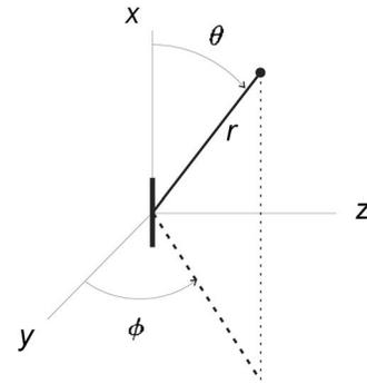
Figure 2. The Cartesian and spherical coordinate systems are shown with the dipole antenna included. The antenna is oriented in the  $x$ -direction. The elevation angle  $\theta$  is between the plane defined by the  $y$ - and  $z$ -axes and the  $x$ -axis ( $yz$ -plane). The azimuth angle  $\phi$  is in the  $yz$ -plane.
