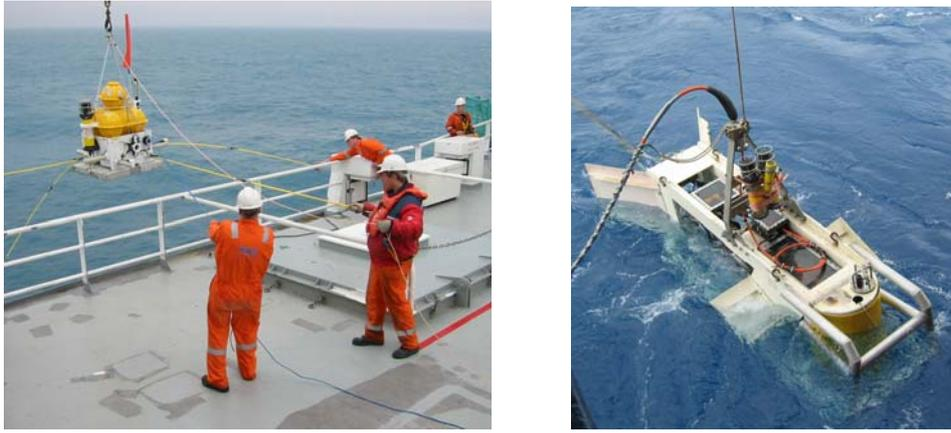
Figure 1: Deployment of receiver and tow fish.
