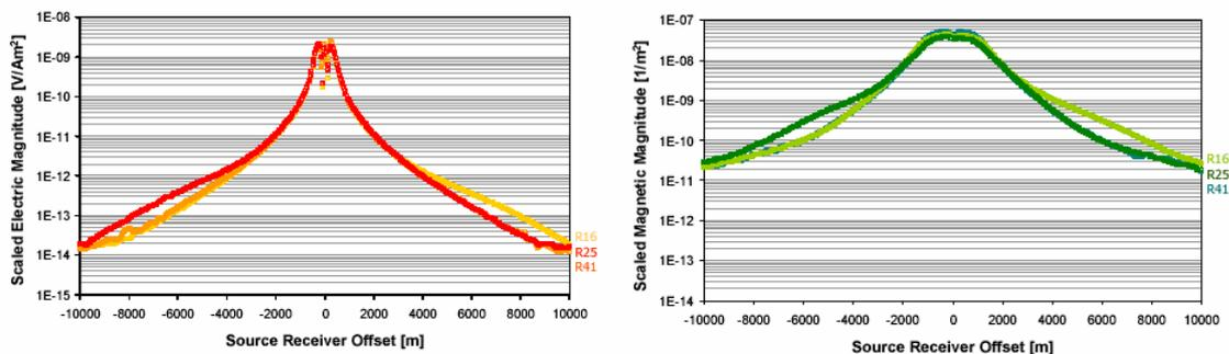
Figure 3: Electric magnitude (left) and magnetic (right) recorded during in- and out-towing for receivers R16, R25 and R41 (0.25 Hz square wave).
