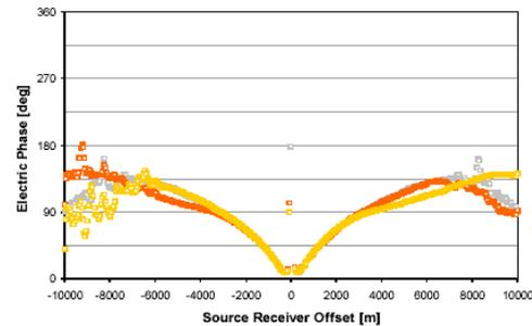
Figure 5: Electric phase versus source receiver offset for receivers R16, R25 and R41 for both in- and out-towing (0.25 Hz).
