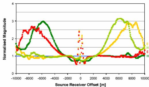
Figure 4: Normalized electric and magnetic magnitudes for receivers R16 and R25 for both in- and out-towing (0.25 Hz). Reference receiver is R41 out-towing.
