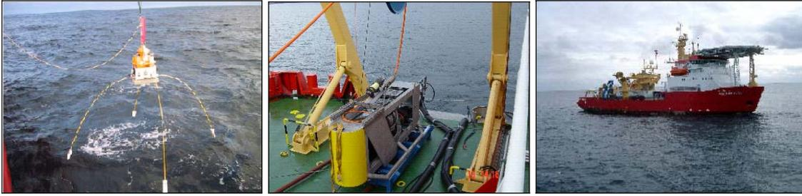
Figure 1: The left picture shows the first instrument dropped over Ormen Lange. All instruments have electrodes mounted at the end of each electrode arms, with lengths around 8m, giving two orthogonal electrical channels. The electric field measured at each channel is amplified and converted from analog to digital format before being recorded on an internal storage device. The EM source tow fish is displayed in the middle. The Polar Björn shown to the right was used as survey vessel.
