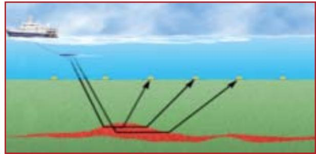
Vessel tows a high-power electromagnetic source while recording the direct, reflected, and refracted signals on the seabed.
