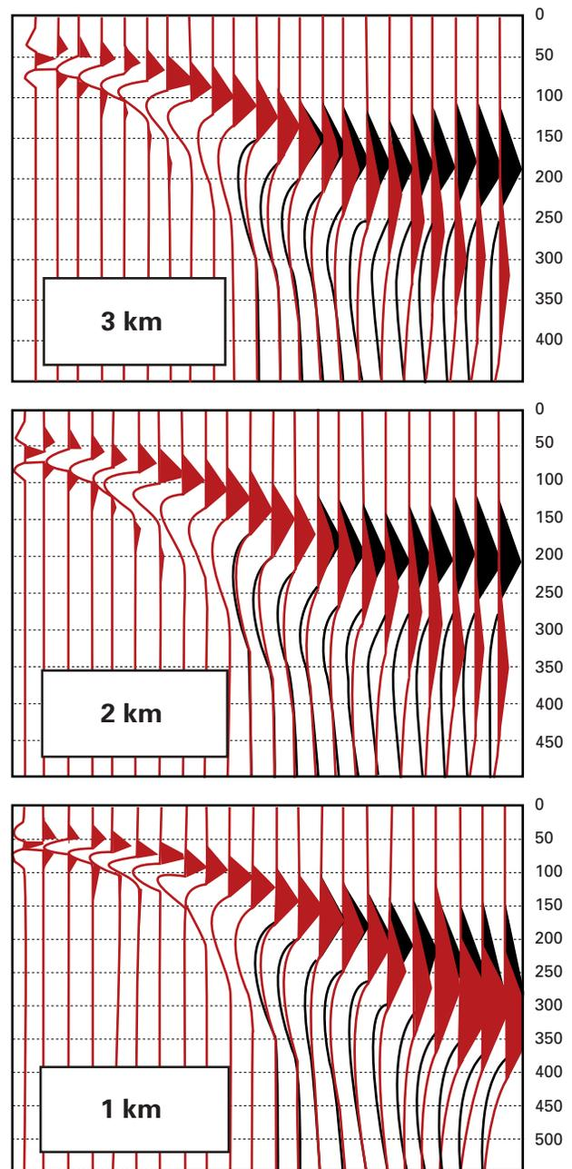
Traces of normalized receiver signals for source-receiver offset 0-4,200 m. Black traces = hydrocarbon-filled reservoir; red traces = water-filled reservoir.
