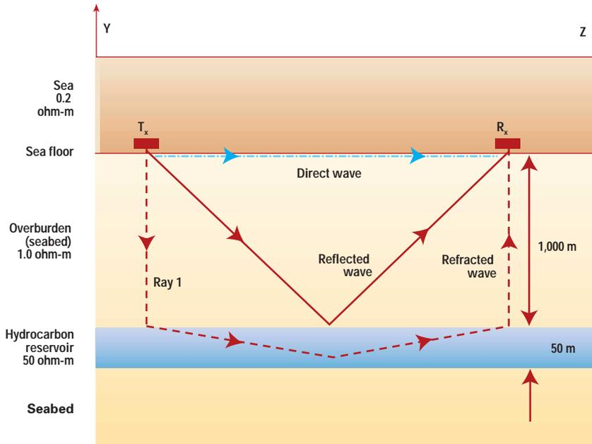
horizontal electric dipole transmitter placed on the sea floor. The complete radial electric field  $E_p$  (the field along the antenna
