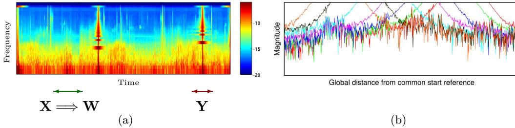
Figure 1: (a) Spectrogram of the data in an electric channel from one of the SBL receivers deployed during the survey described in the text. The time periods selected for training and cleaning have respectively been marked by green and red arrows. (b) Cleaning period magnitude vs offset plots for an electric channel of seven of the SBL receivers deployed during the survey described in the text.
