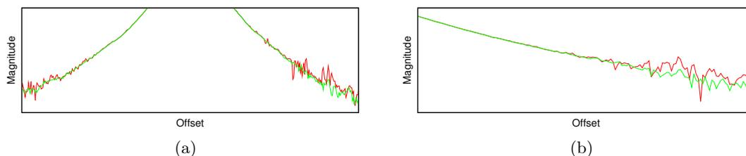
Figure 2: Magnitude vs offset plots for an electric channel of two different SBL receivers deployed during the survey described in the text before (red) and after (green) MT signal removal.
