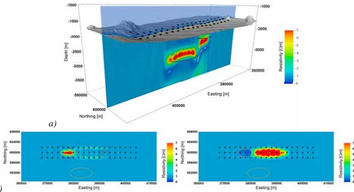
**Figure 3** Denser 3D grid dataset inversion result and receiver positions. a) Vertical section along resistors A and B with polygons that indicate outline of true model resistors. b) Depth slices at 2500 m and 2900 m.
