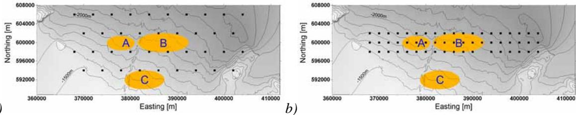
**Figure 1** True model resistors and bathymetry with receiver layout for a) scanning survey and b) denser 3D grid. Resistor depth below sea surface (approximate depth below seafloor): A 2500 m (850 m), B 3000 m (1300 m), C 2800 m (1300 m).
