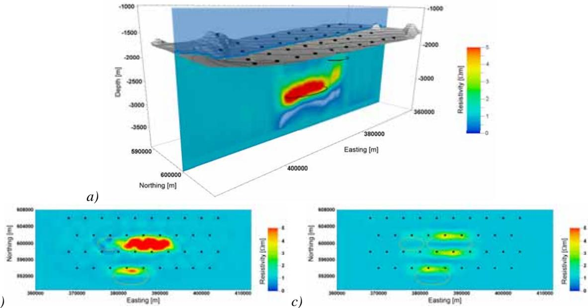
**Figure 2** Scanning dataset inversion including azimuth data in a) and b), and using inline data only in c). Fig. a) shows vertical section along resistors A and B with black polygons to outline the true model resistors, and b) shows a depth slice at 3000 m. c) Depth slice at 3200 m (strongest response).
