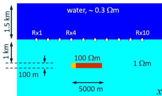
Figure 1: A 2.5D marine CSEM model used for the 4D study, as proposed by Orange *et al.*, 2009. A 100 m thick oil reservoir with resistivity  $100 \Omega\text{m}$  is buried 1 km below the seabed. It is flooded from the left edge and reduction in its volume is picked up by CSEM response measured by 10 seabed receivers spaced by 2 km.
