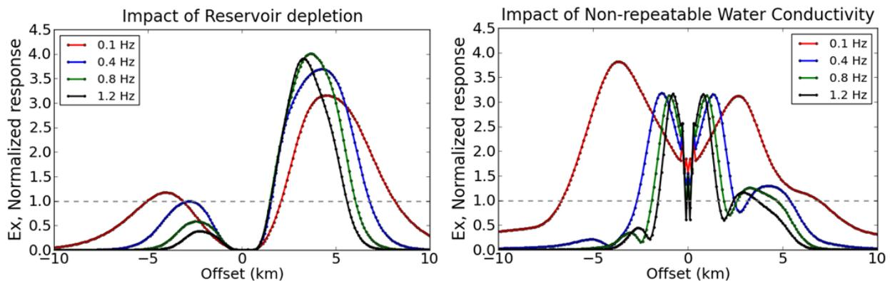
Figure 2: CSEM response resulting from a 4% depletion of the reservoir (left) and from a 4.5% variation of seawater conductivity (right). The response is recorded for receiver Rx4 placed above the depletion region (see Fig.1) and normalized to data uncertainty (dashed line shows the noise level). Variation of water conductivity strongly affects CSEM data and can mask the time-lapse response.
