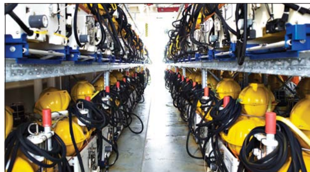
Figure 2 Up to 200 receivers can be kept aboard EMGS's high-capacity 3D EM surveying vessels. More receivers means larger and more complex surveys, and more data points per km 2 for improved 3D data coverage.
